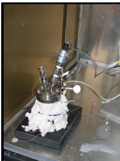
Lab batch reactor 100 ml open volume (rate: 3L H 2 /hr for 0.5hrs)
