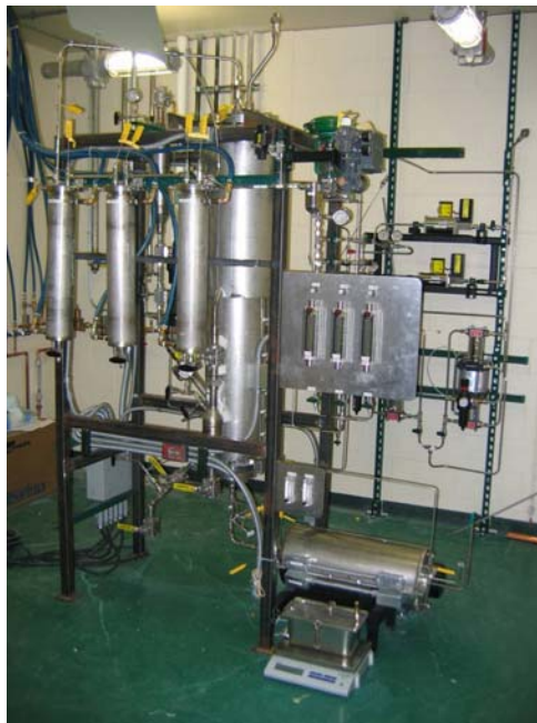
Figure 12. Prototype 10 kg H 2 /day solid biomass reactor
